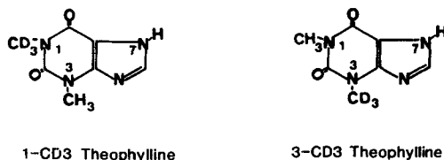
Figure 1 : Structure of the trideuteromethyl-theophylline molecules (for clearness of presentation ^2H was noted D in figures).
